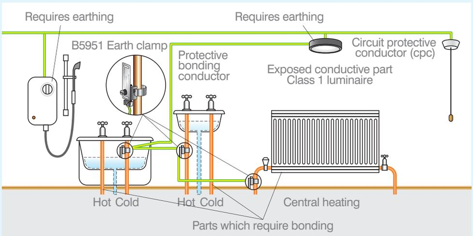
**Earthing Conductor** A protective conductor connecting the main earthing terminal of an installation to an earth electrode or other means of earthing.
